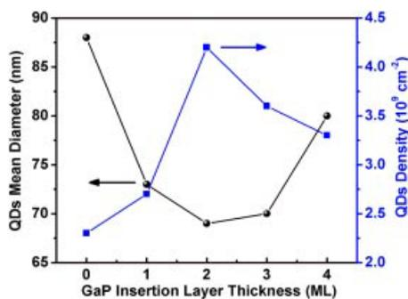
**Figure 3.** The average diameter and density of InP QD as a function of GaP insertion layer thickness.
