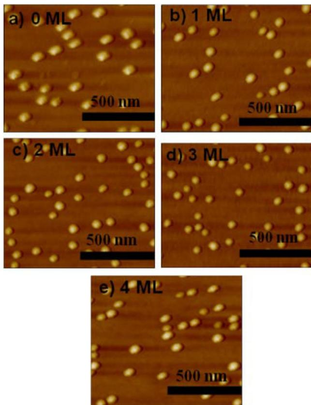
**Figure 2.** Typical ( $1\ \mu\text{m} \times 1\ \mu\text{m}$ ) scan range AFM images of InP QDs embedded in InGaP barrier with (a) 0 ML, (b) 1 ML, (c) 2 ML, (d) 3 ML and (e) 4 ML GaP layers.
