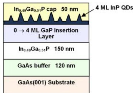
**Figure 1.** Schematic diagram of the vertical layer structure of InP QDs embedded in InGaP barrier grown on (001) GaAs substrate.
