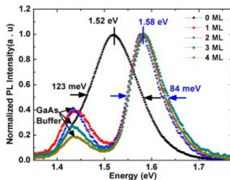
**Figure 4.** The room temperature PL spectra of the InP QDs grown on the InGaP barrier with 0–4 ML thick GaP insertion layer between the InP QDs and the InGaP barrier.
